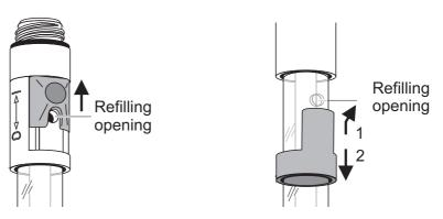
• Remove the watering cap from the electrode tip. Possible salt deposits in the area of the watering cap do not affect the measuring characteristics and can easily be removed with deionized water.
